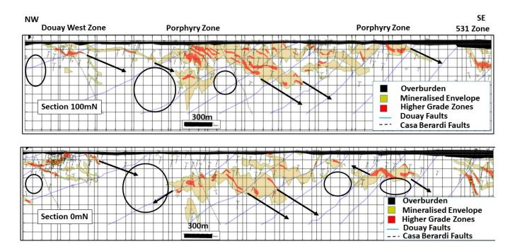
Long section @106, looking NNE. Top is section 100N, bottom is section 0N. Mineralised zones deepen southwards.
