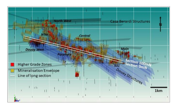
Figure 1: 2D representation of 3D structural model showing distribution of higher-grade mineralized zones (red), within lower-grade envelope (yellow), controlled by the two main sets of structures: the E-W Casa Berardi set (grey) and the NW-SE Douay set (blue). Note trace of longitudinal sections 100mN and 0mN as also shown in Fig. 2 below).
