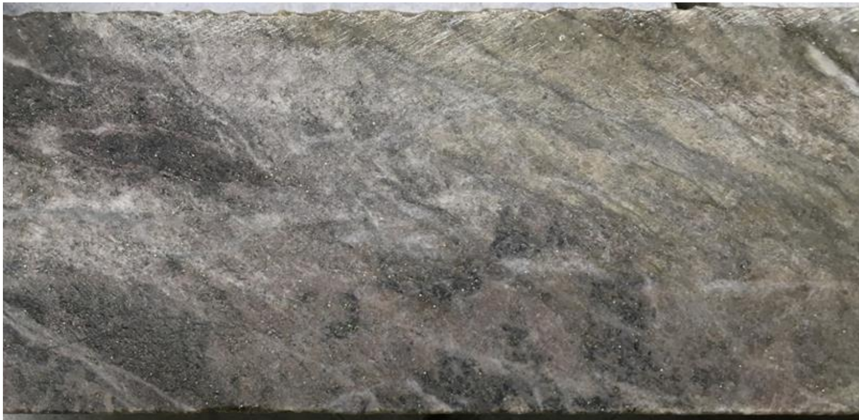
Sheared basalt with diffuse syenite injections and carbonate veinlets. Patchy carbonate-sericite-hematite alteration; 5% fine to medium-grained pyrite. From interval 403-404m that gave 9.78 g/t Au. NQ core = 47.6mm diameter
