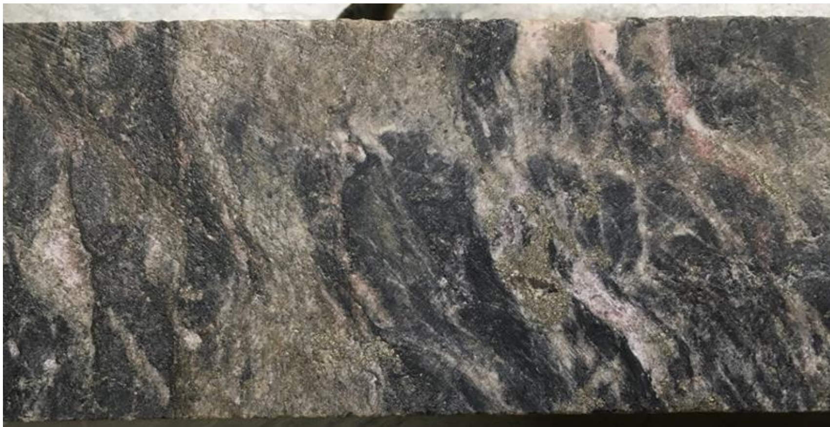
Sheared basalt with syenite injections and carbonate veinlets. Patchy carbonate-sericite-hematite alteration; 5% fine to medium-grained pyrite. From interval 398-399m that gave 5.9 g/t Au. NQ core = 47.6mm diameter
