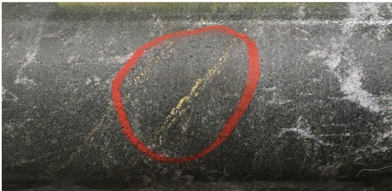
Plate 2: Gold-rich veinlets within altered basalts in hole DO-21-302 at about 508.5 m, forming part of the sample grading 1.0 m of 21.7 g/t Au. Core diameter is 47.6 mm.
