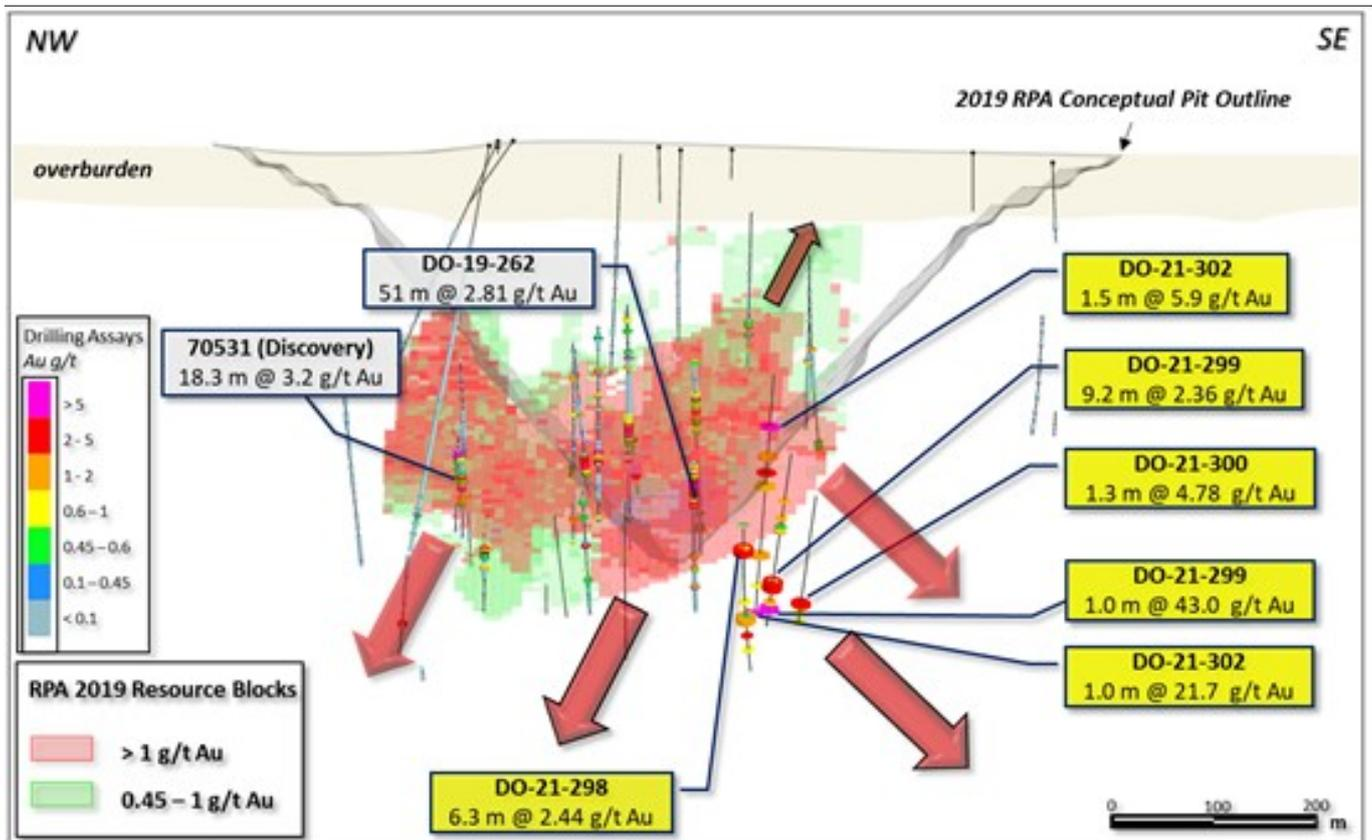
Figure 2: NE-looking longitudinal section (100 m total corridor width) through the 531 Zone showing two possible sub-orthogonal plunges, including the SE extension drilled by holes reported in this PR.
