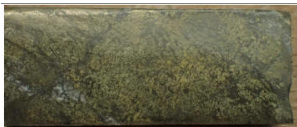
Plate 2: Semi-massive pyrite cut by iron carbonate veinlet (lower left) at 354.9 m in EM-14-001, part of a 1 m sample interval that gave 13.7 g/t Au.
