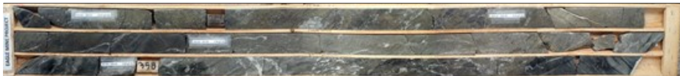
Plate 1: Core box containing the main mineralized interval in hole EM-14-001 from 354.6 to 359.1 m downhole, showing abundant pyrite as well as white iron-carbonate veinlets.
