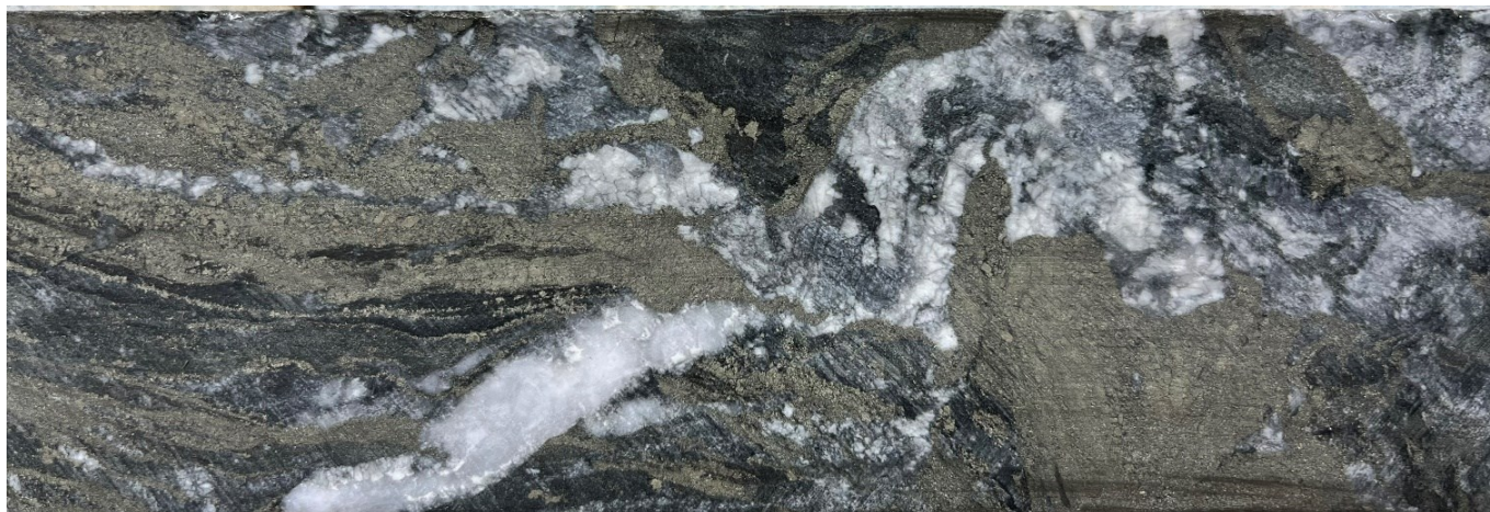
Plate 1: Semi-massive pyrite with iron-carbonate veinlets at 346.5 m downhole in drill hole EM-22-005 (#5 pierce point shown on Figure 1); mineralization extends from 346 to 363.5 m downhole. Assays are pending; NQ core (47.6mm diameter)
